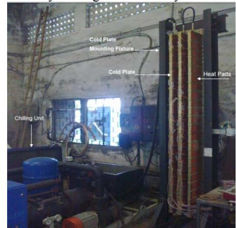
Figure 13 Thermal test of one loop of cold plate
